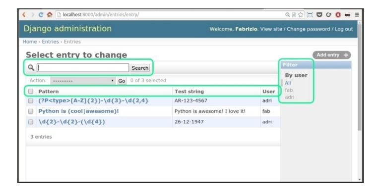
I have highlighted the three parts of this view that we customized in the EntryAdmin class. We can filter by user, we can search and we have all the fields displayed. If you click on a pattern, the edit view opens up.
